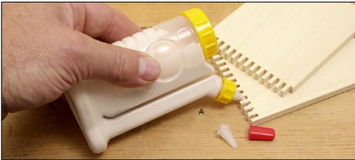
This dripless glue dispenser is ideal for small-scale work. With a gentle squeeze of the bottle, glue is forced through a channel at the bottom of the airtight reservoir and up the spout. This displacement creates a vacuum in the reservoir that siphons excess glue from the spout as you ease your grip, preventing drips. The 4 oz. bottle is supplied with two trimmable nozzles, flat for dispensing a strip of adhesive and conical for
